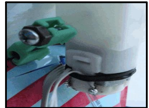
Wires on geared down motor
