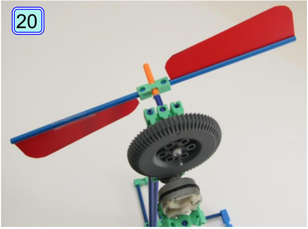
Cut out blade shapes and slide into slit rods
